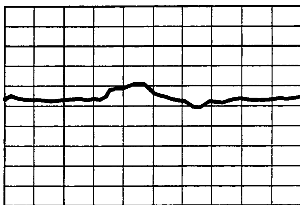
Figure 4-6. Residual FM Signal as displayed on a Spectrum Analyzer
